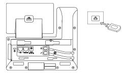
Note: The USB port can also be used to connect other USB devices, such as EXP50, USB headset and so on.
